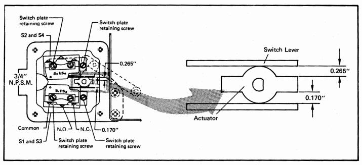
Figure 6-4 Typical Preset Switch Assembly
